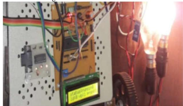
Figure 9: The state of IR sensor during the presence of person When any person is present in a boggie, it is sensed by an IR sensor that only the light turns on. The relay follows this
