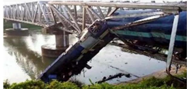
Figure 1: The calamity was caused by a track break.
