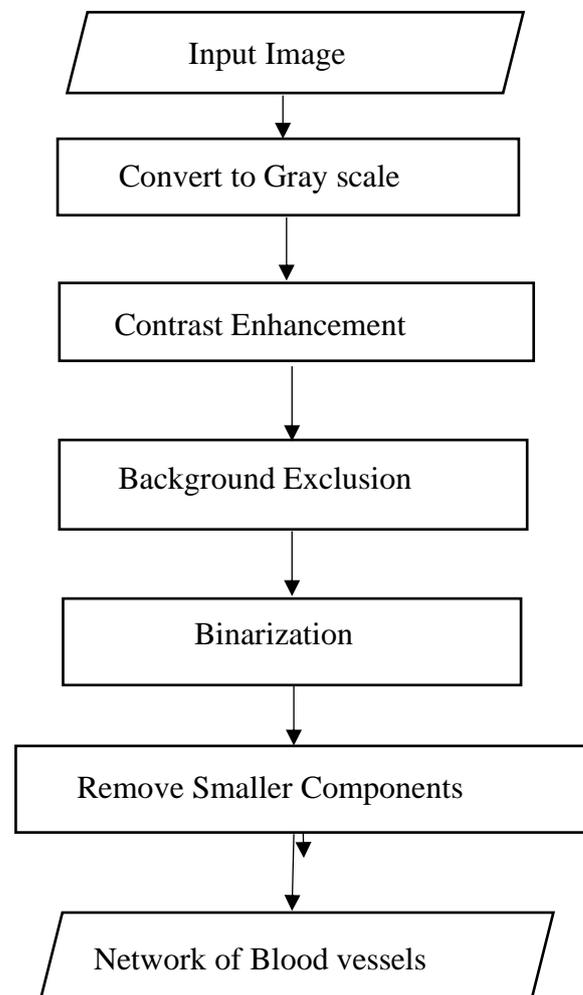
Figure-1: Block Diagram of Retinal Vessel Segmentation
