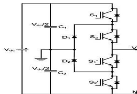
Figure 1: Neutral Point Clamped Inverter
