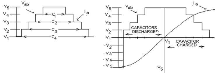
Figure 3: Waveforms Showing Capacitor Charging Profile (a) Voltage and Current in Phase (b) Voltage and Current Are  $90^\circ$  Out of Phase.
