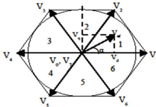
Figure 4: Representation of Rotating Vector in a Complex Plane Space Vector Representation of the Three-Phase Quantity
